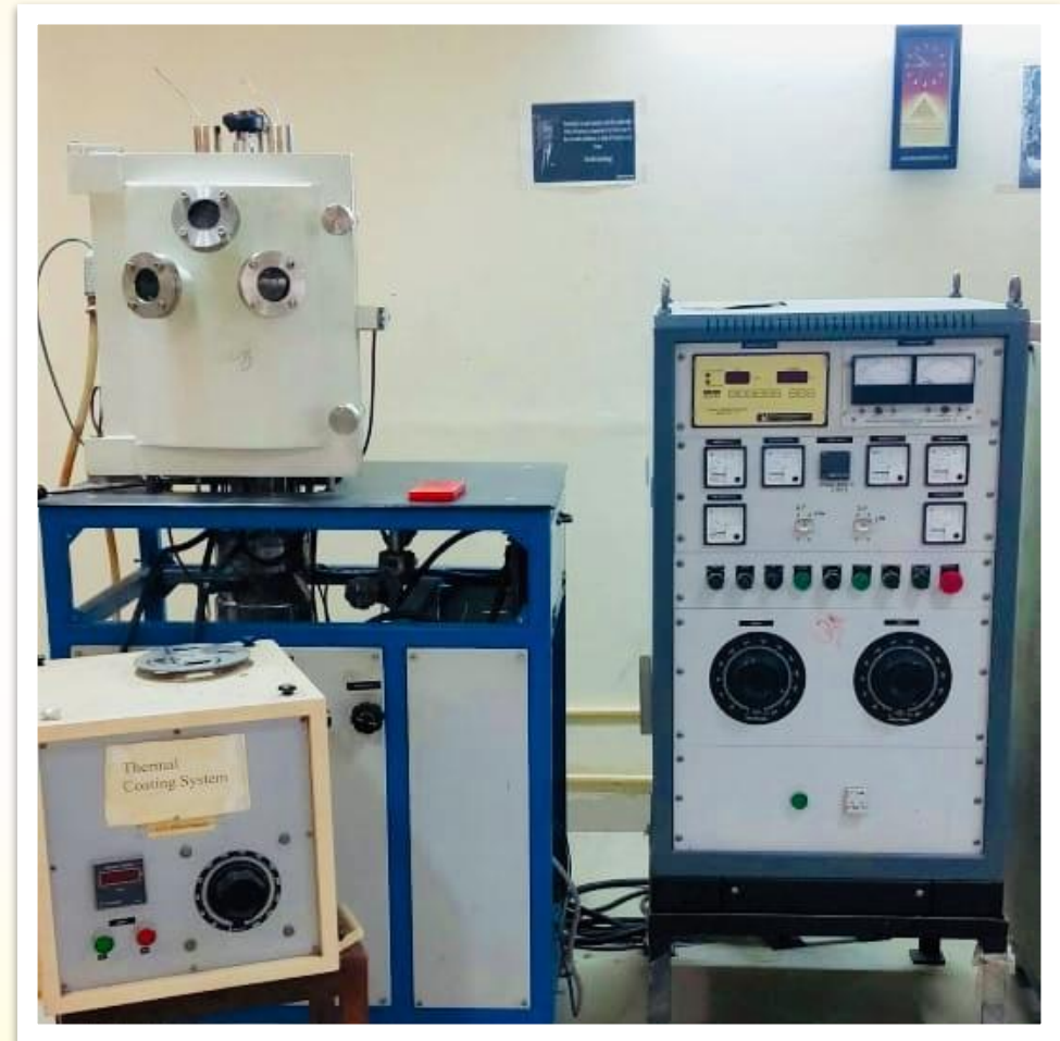
THERMAL VACUUM COATING UNIT
